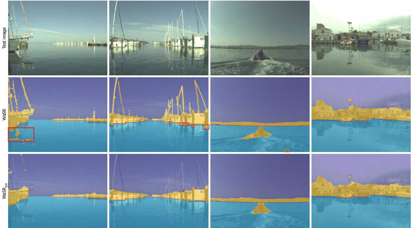
Figure 5: WaSR (fully-supervised) vs. WaSR_{SLR} trained using the proposed scaffolding approach. WaSR often predicts false positive detections on water reflections of obstacles (columns 1 and 2), while WaSR_{SLR} is more robust. WaSR_{SLR} also performs well in difficult scenarios such as wakes (column 3) and heavy reflections (column 4). Best viewed on a screen.
