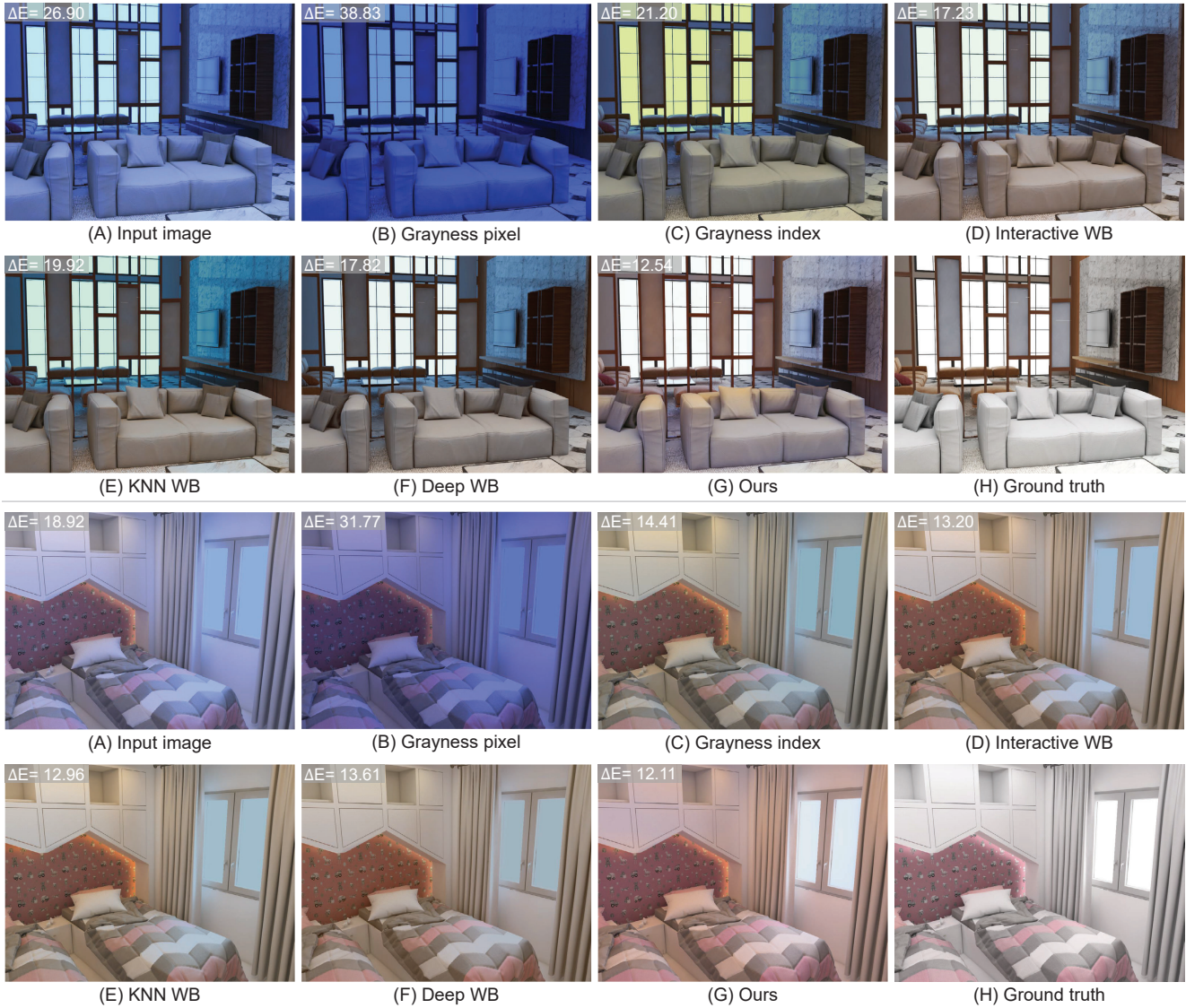
Figure 6: Qualitative comparisons with other AWB methods on our mixed-illuminant evaluation set. Shown are the results of the following methods: gray pixel [16], grayness index [17], interactive WB [4], KNN WB [5], deep WB [3], and our method.
