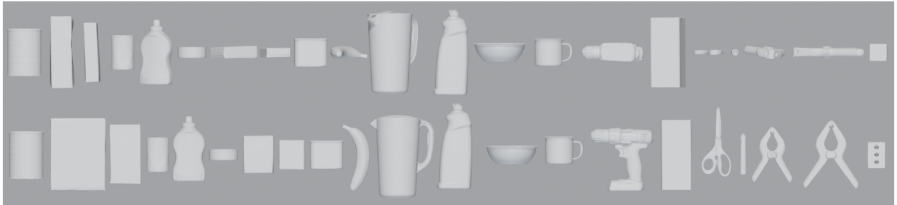
Figure 3. YCB-VIDEO objects in default (top) and our canonical frame (bottom). Objects without a rotational symmetry (banana, pitcher, bleach, mug, driller, scissors) are aligned with respect to their mirror-symmetry plane.
