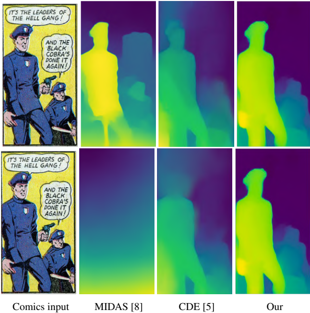
Figure 2: Qualitative comparison of depth estimation on the DCM validation images [7] from our benchmark. (Top Row): Depth predictions on the translated comics images as seen in the main paper. (Bottom Row): Depth predictions on the actual comics images (not translated). We show, from left to right, the input image in the comics domain, the result using the MIDAS [8] model, the result using the CDE [5] model, and Our model (comprising I2I, depth, feature GAN, Laplacian and the text module), respectively. We show that all the methods benefit from the I2I module. Further, we show that our approach can predict depth when applied both to the translated image, as well as the original comics image; while outperforming the baselines in both the scenarios. Cooler colors are farther and warmer colors are nearer (Best viewed in color).
