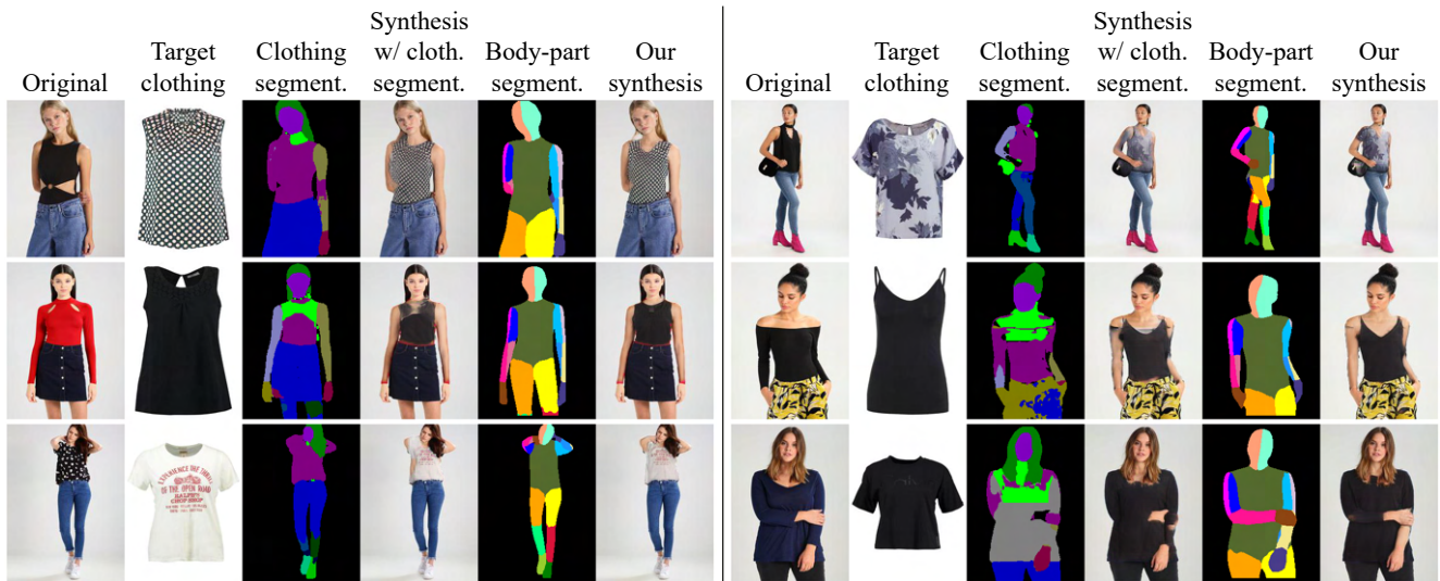
Figure 25. Comparisons of clothing and body-part segmentations and their effect on the synthesis quality of C-VTON on the MPV dataset. The use of clothing segmentations affects sleeve generation, garment edges and arm generation in difficult poses. The figure is best viewed in color and zoomed in.
