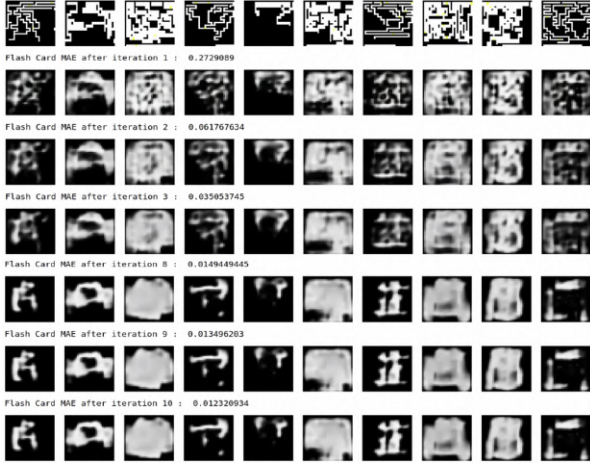
Figure 3. Different iterations of flashcards construction from maze patterns, after training autoencoder on Fashion MNIST
