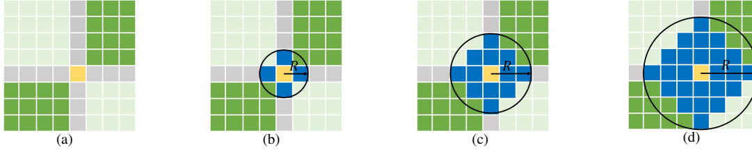
Figure 6. We take a feature map of size 8 \times 8 as an example to illustrate how to decide the radius of the circle. In the first subplot, The dark and light green show the conjugate symmetry property after \mathcal{F}(\cdot) and \text{fftshift}(\cdot) operations, and the yellow square represents the DC component. Subplots (b)-(c) illustrate how to define the radius, and the blue squares are the elements will be summed up in the circle. The radii in (b)-(c) are 1, 2 and 3, respectively.
