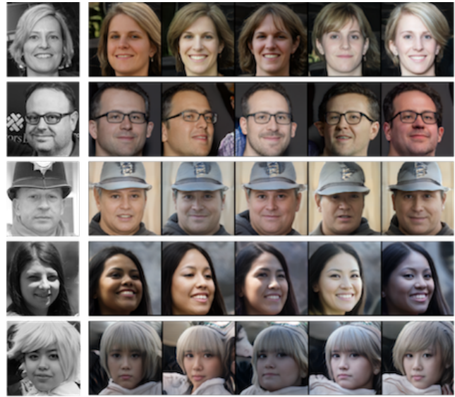
(d) Colourization - First column shows gray-scale image describing desired high-level semantics. Rest columns correspond to images generated when Vgg16 features of the gray-scale version is provided as prior in DISP module.
