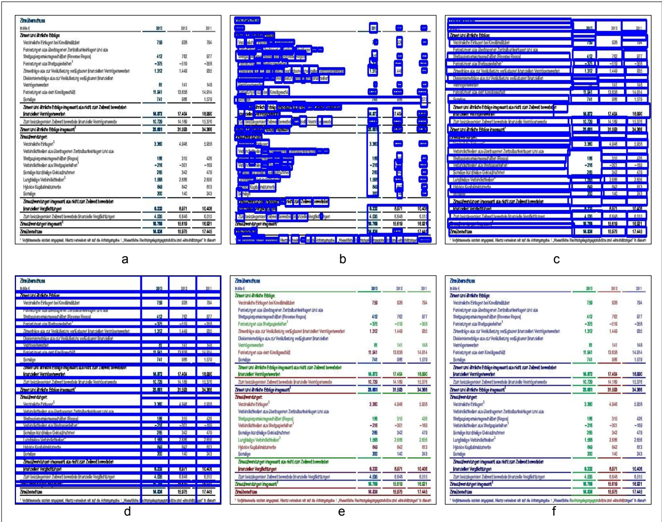
Figure 9. Illustrates visual results of TUCD. (a) original table image, (b) word detection using Tesseract, (c) cell detection using TOD-Net, (d) cell detection using intersection of detected row and column using TOD-Net, (e) cells which are row adjacent using TSR-Net, and (f) cells which are column adjacent using TSR-Net.
