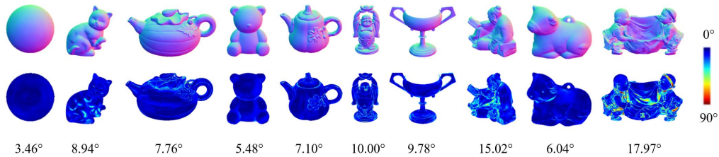
(d) Estimated normals and corresponding error maps using the complete search space.
